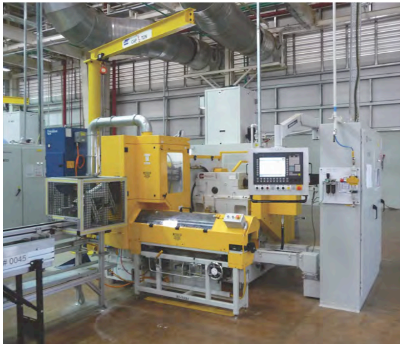
C & B Double Disc Grinding System in Allison’s Facility in Chennai, India
